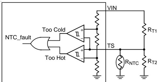
$$R_{T2} = \frac{310R_{TC}R_{TH}}{117R_{TC} - 427R_{TH}}$$
