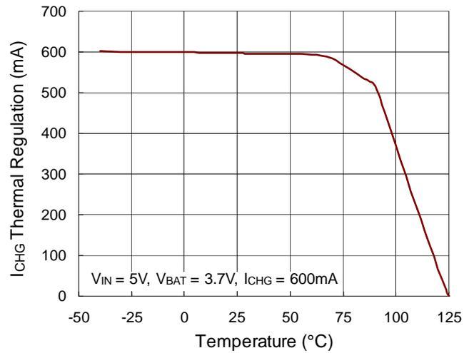
**I<sub>CHG</sub> Thermal Regulation vs. Temperature**
