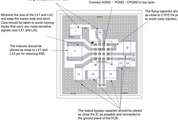
Figure 2. PCB Layout Guide
