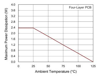
Figure 1. Derating Curve of Maximum Power Dissipation
