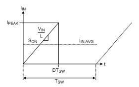
Figure 2. The Buck-Boost Input Signature in BCM
