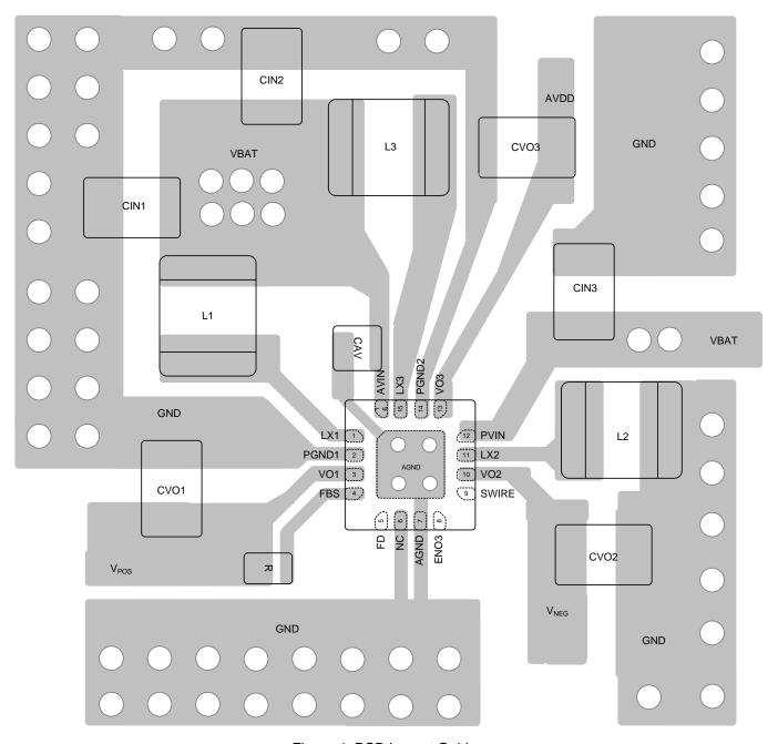
Figure 4. PCB Layout Guide
