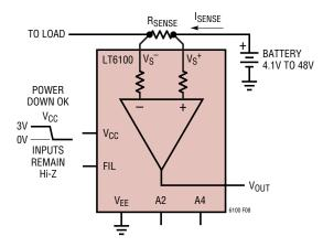
This is the typical configuration for an LT6100, monitoring the load current of a battery. The circuit is powered from a low-voltage supply rail rather than the battery being monitored. A unique benefit of this configuration is that when the LT6100 is powered down, its battery sense inputs remain high impedance, drawing less than 1uA of current. This is due to an implementation of Linear Technology's Over-The-Top® input technique at its front end.
