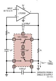
The LTC6943 is used to accurately sample the voltage across the  $1k\Omega$  sense resistor and translate it to a ground reference by charge balancing in the  $1\mu F$  capacitors. The LTC2050 integrates the difference between the sense voltage and the input command voltage to drive the proper current into load.
