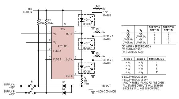
The LTC1921 provides an all-in-one telecom fuse and supply-voltage monitoring function. Three opto-isolated
