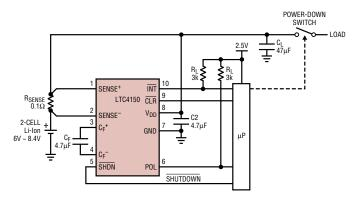
This is the same as the Coulomb Counter circuit, except that the microprocessor clears the integration cycle complete condition with software, so that a relatively slow polling routine may be used.
