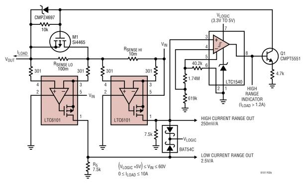
Using two current sense amplifiers with two values of sense resistors is an easy method of sensing current over a wide range. In this circuit the sensitivity and resolution of measurement is 10 times greater with low cur-
