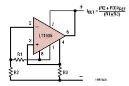
The LT1635 combines an op amp with a 200mV reference. Scaling this reference voltage to a potential across resistor R3 forces a controlled amount of current to flow from the +terminal to the -terminal. Power is taken from the loop.
