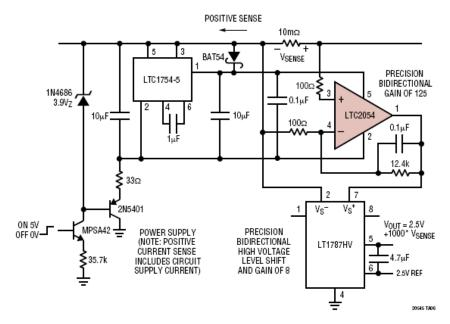
Using a very precise zero-drift amplifier as a pre-amp allows for the use of a very small sense resistor in a high voltage supply line. A floating power supply regulates the voltage across the pre-amplifier on any voltage rail up to the 60V limit of the LT1787HV circuit. Overall gain of this circuit is 1000. A 1mA change in current in either direction through the  $10m\Omega$  sense resistor will produce a 10mV change in the output voltage.
