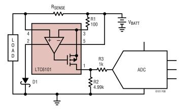
If the output of the LTC6101 is wired to an independently powered device that will effectively short the output to another rail or ground (such as through an ESD protection clamp) during a reverse supply condition, the LTC6101's output should be connected through a resistor or Schottky diode to prevent excessive fault current.
