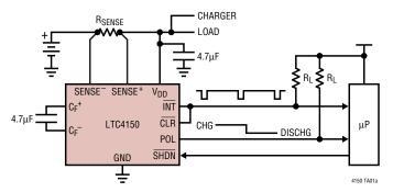
The LTC4150 is a micropower high-side sense circuit that includes a V/F function. Voltage across the sense resistor is cyclically integrated and reset to provide digital transitions that represent charge flow to or from the battery. A polarity bit indicates the direction of the current. Supply potential for the LTC4150 is 2.7V to 8.5V. In the free-running mode (as shown, with CLR & INT connected together) the pulses are approximately  $1\mu s$  wide and around 1Hz full-scale.
