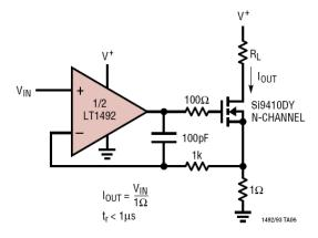
This is a simple controlled current sink, where the op amp drives the NMOSFET gate to develop a match between the  $1\Omega$  sense resistor drop and the VIN current command. Since the common-mode voltage seen by the op amp is near ground potential, a "single-supply" or Rail-to-Rail type is required in this application.
