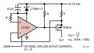
This is a simple current-source configuration where the op amp servos to establish a match between the drop on the sense resistor and that of the 1.2V reference. This particular op amp includes a shutdown feature so the current source function can be switched off with a logic command. The  $2k\Omega$  pull-up resistor assures the output MOSFET is off when the op amp is in shutdown mode.
