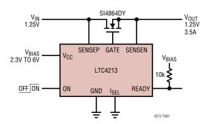
The LTC4213 provides protection and automatic circuit breaker action by sensing Drain-to-Source voltage-drop across the NMOSFET. The sense inputs have a Rail-to-Rail common mode range, so the circuit breaker can protect bus voltages from OV up to 6V. Logic signals flag a trip condition (with the READY output signal) and reinitialize the breaker (using the ON input). The ON input may also be used as a command in a "smart switch" application.
