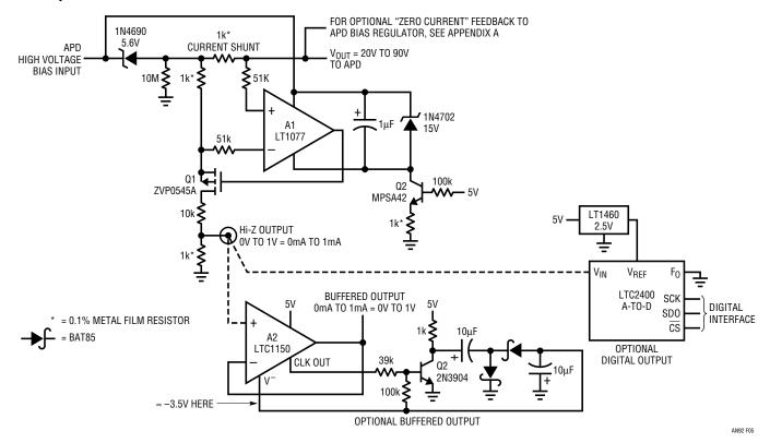
Avalanche Photodiodes, APDs, require a small amount of current from a high voltage supply. The current into the diode is an indication of optical signal strength and must be monitored very accurately. It is desirable to power all of the support circuitry from a single 5V supply.
