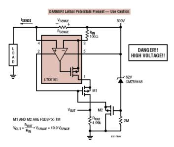
Adding two external Mosfets to hold off the voltage allows the LTC6101 to connect to very high potentials and monitor the current flow. The output current from the LTC6101, which is proportional to the sensed input voltage, flows through M1 to create a ground referenced output voltage.
