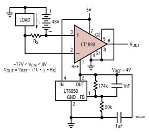
The LT1990 is a wide common-mode range difference amplifier used here to amplify the sense resistor drop by 10. To provide the desired input range when using a single 5V supply, the reference potential is set to approxi-
