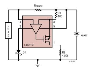
The LTC6101 is not protected internally from external reversal of supply polarity. To prevent damage that may occur during this condition, a Schottky diode should be added in series with  $V^-$ . This will limit the reverse current through the LTC6101. Note that this diode will limit the low voltage performance of the LTC6101 by effectively reducing the supply voltage to the part by  $V_D$ .
