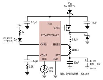
Controlling the current flow in Lithium-Ion battery chargers is essential for safety and extending useful battery life. Intelligent battery charger ICs can be used in fairly simple circuits to monitor and control current, voltage and even battery pack temperature for fast and safe charging.
