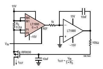
The LT1995 amplifies the sense resistor drop by 5V/V and subtracts that from  $V_{\text{IN}}$ , providing an error signal to an LT1880 integrator. The integrated error drives the PMOSFET as required to deliver the commanded current.
