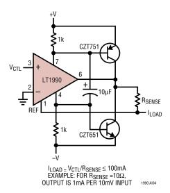
This is a classical Howland bidirectional current source implemented with an LT1990 integrated difference amplifier. The op amp circuit servos to match the RSENSE voltage drop to the input command VCTL. When the load current exceeds about 0.7mA in either direction, one of the boost transistors will start conducting to provide the additional commanded current.
