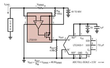
The LTC2433-1 can accurately digitize signal with source impedances up to  $5k\Omega$ . This LTC6101 current sense circuit uses a  $4.99k\Omega$  output resistance to meet this requirement, thus no additional buffering is necessary.
