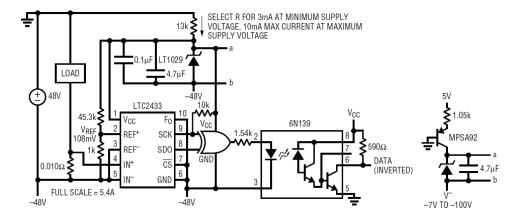
In this circuit an economical ADC is used to acquire the sense resistor voltage drop directly. The converter is powered from a "floating" high-accuracy shunt-regulated supply and is configured to perform continuous conversions. The ADC digital output drives an opto-isolator, level-shifting the serial data stream to ground. For wider supply voltage applications, the 13k biasing resistor may be replaced with an active 4mA current source such as shown to the right. For complete dielectric isolation
