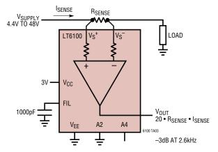
The LT6100 has pin strap connections to establish a variety of accurate gain settings without using external components. For this circuit grounding A2 and leaving A4 open set a gain of 20. Adding one external capacitor to the FIL pin creates a low-pass filter in the signal path. A capacitor of 1000pF as shown sets a filter corner frequency of 2.6KHz.
