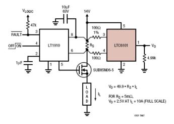
The LT1910 is a dedicated high side MOSFET driver with built in protection features. It provides the gate drive for a power switch from standard logic voltage levels. It provides shorted load protection by monitoring the current flow to through the switch. Adding an LTC6101 to the same circuit, sharing the same current sense resistor, provides a linear voltage signal proportional to the load current for additional intelligent control.
