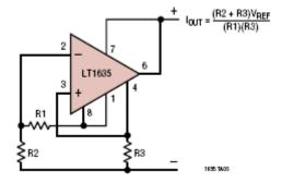
The LT1635 combines an op amp with a 200mV reference. Scaling this reference voltage to a potential across resistor R3 forces a controlled amount of current to flow from the +terminal to the -terminal. Power is taken from the loop.
