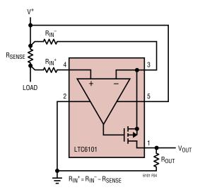
The second input resistor decreases input error due caused by the input bias current. For smaller values of  $R_{\text{IN}}$  this may not be a significant consideration.
