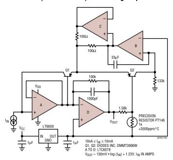
Using precision quad amplifiers like the LTC6079, ( $10\mu V$  offset and <1pA bias current) allow for very wide range current sensing. In this circuit a six decade range of current pulled from the circuit input terminal is converted to an output voltage in logarithmic fashion increasing 150mV for every decade of current change.
