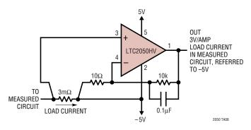
This configuration is basically a standard non-inverting amplifier. The op amp used must support common-mode operation at the lower rail and the use of a Zero-Drift type (as shown) provides excellent precision. The output of this circuit is referenced to the lower Kelvin contact, which could be ground in a single-supply application. Small-signal range is limited by  $V_{OL}$  for single-supply designs. Scaling accuracy is set by the quality of the user-selected resistors.
