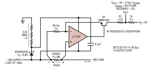
This amplifier configuration is essentially the complementary implementation to the classic high-side configuration. The op amp used must support common-mode operation at its lower rail. A "floating" shunt-regulated local supply is provided by the Zener diode, and the transistor provides metered current to an output load resis-
