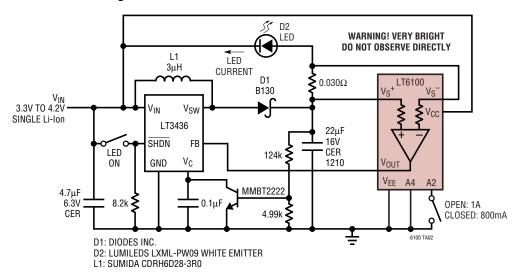
The LT6100 is configured for a gain of either 40V/V or 50V/V depending on whether the switch between A2 and  $V_{EE}$  is closed or not. When the switch is open (LT6100 gain of 40V/V), 1A is delivered to the LED. When the switch is closed (LT6100 gain of 50V/V), 800mA is deliv-
