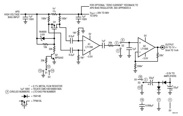
Avalanche Photodiodes, APDs, require a small amount of current from a high voltage supply. The current into the diode is an indication of optical signal strength and must be monitored very accurately. It is desirable to power all of the support circuitry from a single 5V supply.
