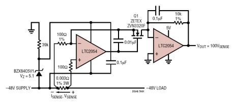
The first stage amplifier is basically a complementary form of the "classic" high-side current sense, designed to operate with telecom negative supply voltage. The Zener forms an inexpensive "floating" shunt-regulated supply for the first op amp. The N-MOSFET drain delivers a metered current into the virtual ground of the second stage, configured as a trans-impedance amplifier (TIA). The second op amp is powered from a positive supply
