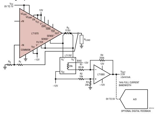
The LT1970 is a 500mA power amplifier with voltage programmable output current limit. Separate DC voltage inputs and an output current sensing resistor control the maximum sourcing and sinking current values. These control voltages could be provided by a D-to-A Converter
