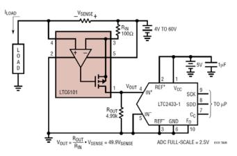
The LTC2433-1 can accurately digitize signal with source impedances up to  $5k\Omega$ . This LTC6101 current sense circuit uses a  $4.99k\Omega$  output resistance to meet this requirement, thus no additional buffering is necessary.
