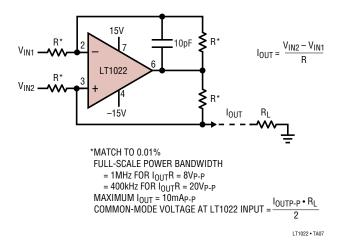
This is a variation on the Howland configuration, where load current actually passes through a feedback resistor as an implicit sense resistance. Since the effective sense resistance is relatively large, this topology is appropriate for producing small controlled currents.
