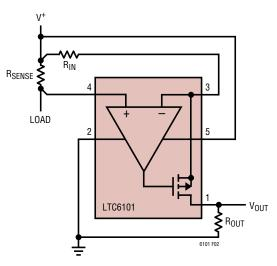
Kelvin connection of the IN– and IN+ inputs to the sense resistor should be used in all but the lowest power applications. Solder connections and PC board interconnections that carry high current can cause significant error in measurement due to their relatively large resistances. By isolating the sense traces from the high current paths, this error can be reduced by orders of magnitude. A sense resistor with integrated Kelvin sense terminals will give the best results.
