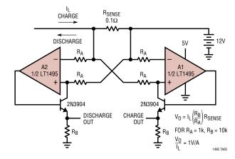
One LT1495 dual op-amp package can be used to establish separate charge and discharge current monitoring outputs. The LT1495 features Over-the-Top operation allowing the battery potential to be as high as 36V with only a 5V amplifier supply voltage.
