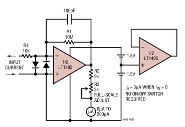
A floating amplifier circuit converts a full-scale 200nA flowing in the direction indicated at the inputs to 2V at the output of the LT1495. This voltage is converted to a current to drive a  $200\mu A$  meter movement. By floating the power to the circuit with batteries, any voltage potential at the inputs are handled. The LT1495 is a micropower op amp so the quiescent current drain from the batteries is very low and thus no on/off switch is required.
