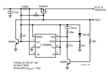
The LT1620I current sense amplifier is used to detect an over-current condition and shut off a P-MOSFET load switch. A fault flag is produced in the over-current condition and a self-reset sequence is initiated.
