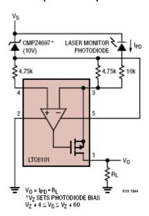
Current through a photodiode with a large reverse bias potential is converted to a ground referenced output voltage directly through an LTC6101. The supply rail can be as high as 70V. Gain of the I to V conversion, the transimpedance, is set by the selection of resistor  $R_{\rm I}$ .
