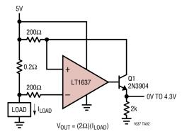
This circuit uses generic devices to assemble a function similar to an LTC6101. A Rail-to-Rail Input type op amp is required since input voltages are right at the upper rail. The circuit shown here is capable of monitoring up to 44V applications. Besides the complication of extra parts, the  $V_{OS}$  performance of op amps at the supply is generally not factory trimmed, thus less accurate than other solutions. The finite current gain of the bipolar transistor is a small source of gain error.
