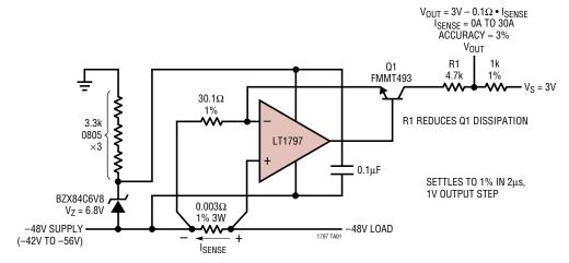
This amplifier configuration is essentially the complementary implementation to the classic high-side configuration. The op amp used must support common-mode operation at its lower rail. A "floating" shunt-regulated local supply is provided by the Zener diode, and the transistor provides metered current to an output load resis-
