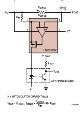
The HV version of the LTC6101 can operate with a total supply voltage of 105V. Current flow in high supply voltage rails can be monitored directly or in an isolated fashion as shown in this circuit. The gain of the circuit and the level of output current from the LTC6101 depends on the particular opto-isolator used.
