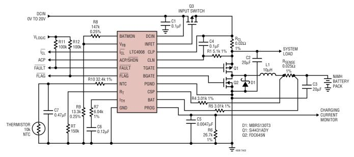
The LTC4008 is a complete NiMH battery pack controller. It provides automatic switchover to battery power when the external DC power source is removed. When power is
