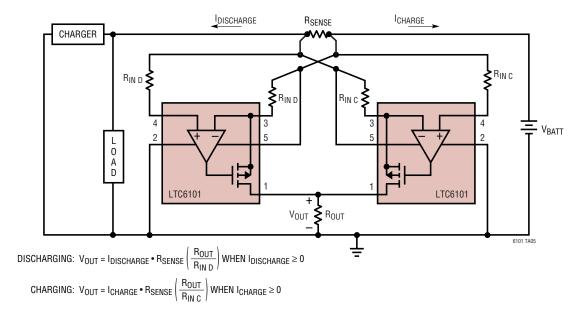
The high impedance current source outputs of two LTC6101's can be directly tied together. In this circuit the voltage at  $V_{OUT}$  continuously represents the absolute
