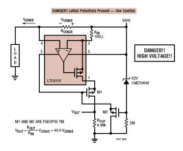
Adding two external Mosfets to hold off the voltage allows the LTC6101 to connect to very high potentials and monitor the current flow. The output current from the LTC6101, which is proportional to the sensed input voltage, flows through M1 to create a ground referenced output voltage.
