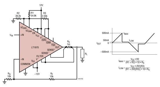
The LT1970 provides current detection and limiting features built-in. In this circuit, the logic flags that are produced in a current-limiting event are connected in a feedback arrangement that in turn reduces the current limit
