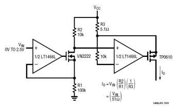
A basic high-side current source is implemented at the output, while an input translation amplifier section provides for flexible input scaling. A Rail-to-Rail input capability is required to have both amplifiers in one package, since the input stage has common-mode near ground and the second section operates near  $V_{\rm CC}$ .
