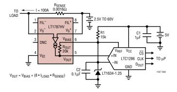
While the LT1787 is able to provide a bidirectional output, in this application the economical LTC1286 is used to digitize a unidirectional measurement. The LT1787 has a nominal gain of eight, providing a 1.25V full-scale output at approximately 100A of load current.
