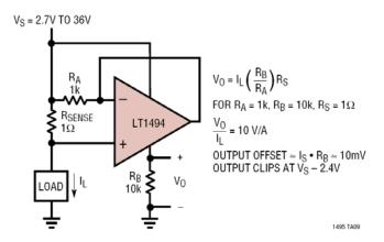
This circuit takes advantage of the microampere supply current and Rail-to-Rail input of the LT1494. The circuit is simple because the supply draw is essentially equal to the load current developed through  $R_{\text{A}}$ . This supply current is simply passed through  $R_{\text{B}}$  to form an output voltage that is appropriately amplified.
