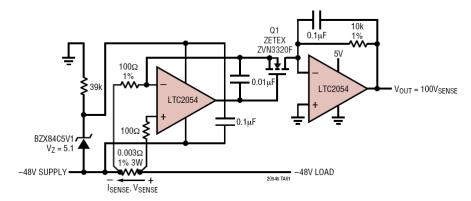
The first stage amplifier is basically a complementary form of the "classic" high-side current sense, designed to operate with telecom negative supply voltage. The Zener forms an inexpensive "floating" shunt-regulated supply for the first op amp. The N-MOSFET drain delivers a metered current into the virtual ground of the second stage, configured as a trans-impedance amplifier (TIA). The second op amp is powered from a positive supply
