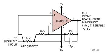
This configuration is basically a standard non-inverting amplifier. The op amp used must support common-mode operation at the lower rail and the use of a Zero-Drift type (as shown) provides excellent precision. The output of this circuit is referenced to the lower Kelvin contact, which could be ground in a single-supply application. Small-signal range is limited by  $V_{OL}$  for single-supply designs. Scaling accuracy is set by the quality of the user-selected resistors.
