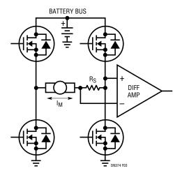
Many of the newer electric drive functions, such as steering assist, are bidirectional in nature. These functions are generally driven by H-bridge MOSFET arrays using pulsewidth-modulation (PWM) methods to vary the commanded torque. In these systems, there are two main purposes for current monitoring. One is to monitor the current in the load, to track its performance against the desired command (i.e., closed-loop servo law), and another is for fault detection and protection features.
