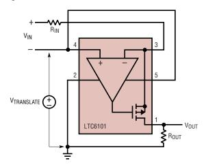
This is a convenient usage of the LTC6101 current sense amplifier as a high voltage level translator. Differential voltage signals riding on top of a high common mode voltage (up to 105V with the LTC6101HV) get converted to a current, through  $R_{\text{IN}}$ , and then scaled down to a ground referenced voltage across  $R_{\text{OUT}}$ .
