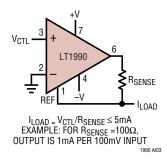
The LT1990 is a differential amplifier with integrated precision resistors. The circuit shown is the classic Howland current source, implemented by simply adding a sense resistor.
