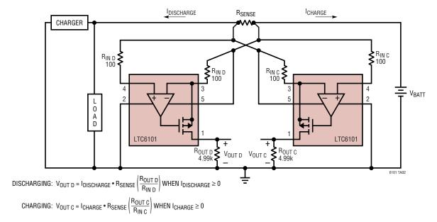
In this circuit the outputs are enabled by the direction of current flow. The battery current when either charging or discharging enables only one of the outputs. For example when charging, the  $V_{OUT}$  D signal goes low since the output MOSFET of that LTC6101 turns completely off
