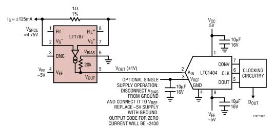
In this circuit, split supply operation is used on both the LT1787 and LT1404 to provide a symmetric bidirectional measurement. In the single-supply case, where the
