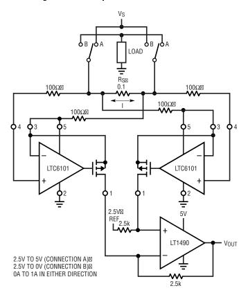
Two LTC6101's are used to monitor the current in a load in either direction. Using a separate rail-to-rail op amp to combine the two outputs provides a single ended output. With zero current flowing the output sits at the reference potential, one-half the supply voltage for maximum output swing or 2.5V as shown. With power supplied to the load through connection A the output will move positive between 2.5V and Vcc. With connection B the output moves down between 2.5V and 0V.
