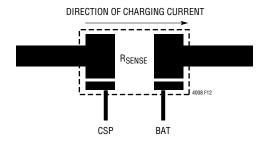
In any high current, >1Amp, application, Kelvin contacts to the sense resistor are important to maintain accuracy. This simple illustration from a battery charger application shows two voltage-sensing traces added to the pads of the current sense resistor. If the voltage is sensed with high impedance amplifier inputs, no IxR voltage drop errors are developed.
