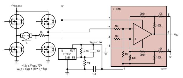
The LT1990 is a difference amplifier that features a very wide common mode input voltage range that can far exceed its own supply voltage. This is an advantage to reject transient voltages when used to monitor the current in a full bridge driven inductive load such as a motor. The LT6650 provides a voltage reference of 1.5V to bias up
