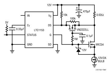
The inrush current created by a lamp during turn-on can be 10 to 20 times greater than the rated operating current. This circuit shifts the trip threshold of an LTC1153 Electronic Circuit Breaker up by a factor of 11:1 (to 30A) for 100ms while the bulb is turned on. The trip threshold then drops down to 2.7A after the inrush current has subsided.
