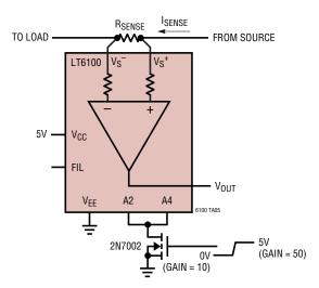
Instead of having fixed gains of 10, 12.5, 20, 25, 40, and 50, this circuit allows selecting between two gain settings. An NMOSFET switch is placed between the two gain-setting terminals (A2, A4) and ground to provide selection of gain = 10 or gain = 50, depending on the state of the gate drive. This provides a wider current measurement range than otherwise possible with just a single sense resistor.
