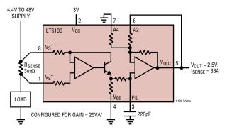
High current sensing on a high voltage supply rail is easily accomplished with the LT6100. The sense amplifier is biased from a low 3V supply and pin-strapped to a gain of 25V/V to output a 2.5V full scale reading of the current flow. A capacitor at the FIL pin to ground will filter out noise of the system (220pF produces a 12KHz low pass corner frequency).
