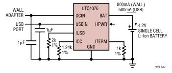
Just a few external components are required for this single Li-lon cell charger. Power for the charger can come from a wall adapter or a computer's USB port.
