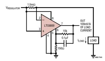
The low offset error of the LTC6800 allows for unusually low sense resistance while retaining accuracy.
