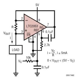
The ultra-precise LTC2053 instrumentation amplifier is configured to servo the voltage drop on sense resistor R to match the command  $V_{\text{C}}$ . The LTC2053 output capability limits this basic configuration to low current applications.
