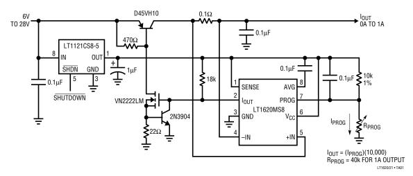
The current output can be controlled by a variable resistor ( $R_{PROG}$ ) connected from the PROG pin to ground on the LT1620. The LT1121 is a low-dropout regulator that keeps the voltage constant for the LT1620. Applying a
