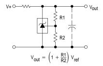
Figure 19. High Current Shunt Regulator
