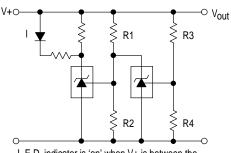
L.E.D. indicator is 'on' when V+ is between the upper and lower limits.
