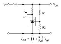
Figure 20. Output Control for a Three–Terminal Fixed Regulator
