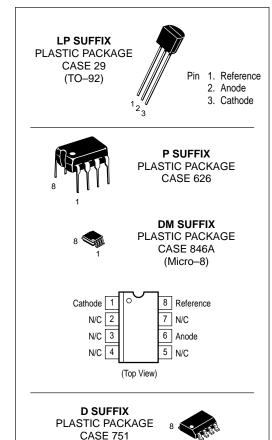
SOP–8 is an internally modified SO–8 package. Pins 2, 3, 6 and 7 are electrically common to the die attach flag. This internal lead frame modification decreases power dissipation capability when appropriately mounted on a printed circuit board. SOP–8 conforms to all external dimensions of the standard SO–8 package.
