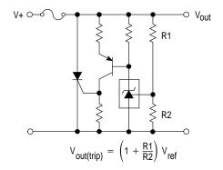
Figure 26. Voltage Monitor
