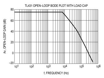
With three poles, this system is unstable. The only hope for stabilizing this circuit is to add a zero. However, that can only be done by adding a series resistance to the output capacitance, which will reduce its effectiveness as a noise filter. Therefore, practically, in reference voltage applications, the best solution appears to be to use a smaller value of capacitance in low noise applications or a very large value to provide noise filtering and a dominant pole rolloff of the system.
