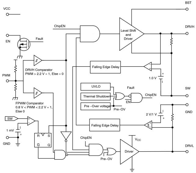
Figure 1. Internal Block Diagram
